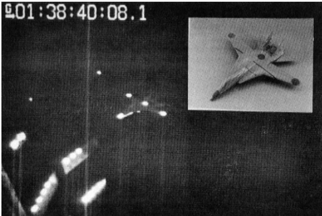
Figure 4. View from one triangulation camera in the spin tunnel.
