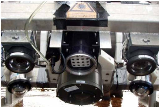
Figure 4. Detail of the 16 laser array mounted between the stereo-video cameras.
