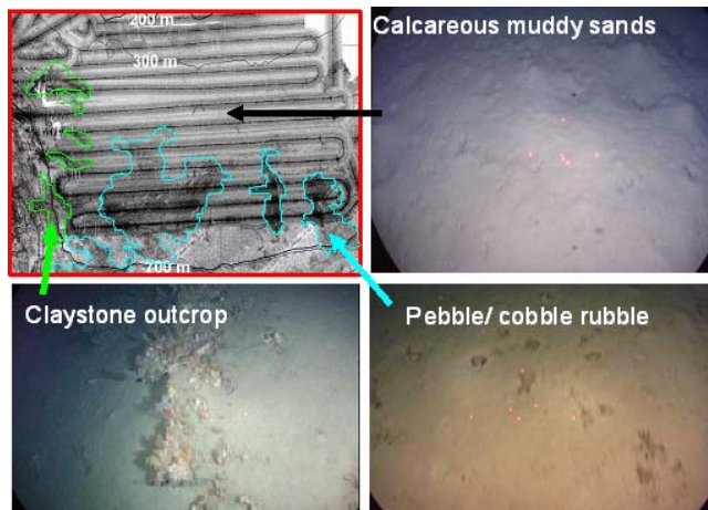
Figure 8. Verification of acoustic terrains by video imagery at canyon edge
