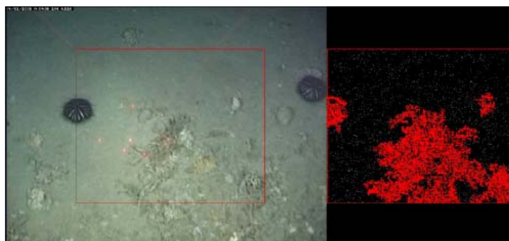
Figure 7. Example of candidate regions detected from motion analysis.
