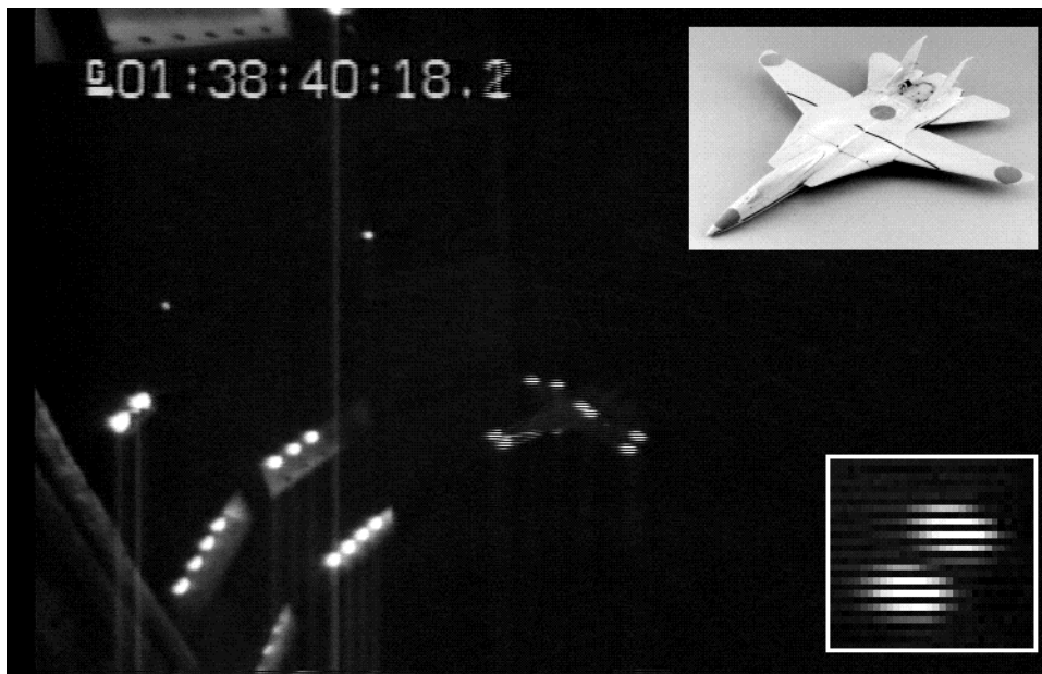
Figure 2. Full frame CCD camera image of a spin tunnel model with (inset upper) the actual model and (inset lower) the effect of motion on one of the retro-reflective targets.
