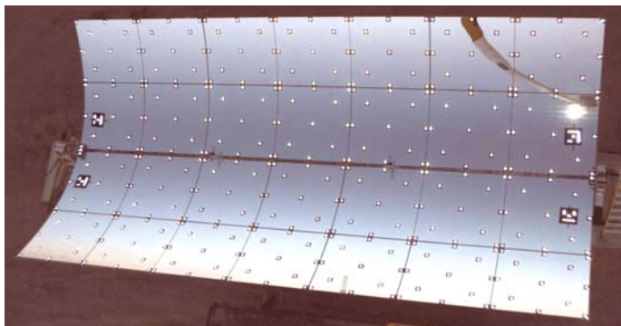
Figure 3: EuroTrough collector element with measurement targets on the concentrator mirrors
