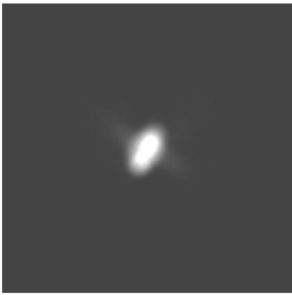
Figure 16: Image of the expected light distribution at the 370 mm focal point of the mirror facet
