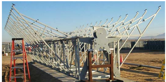
Figure 1: Space frame of a EuroTrough module with measurement targets on the mirror support points
